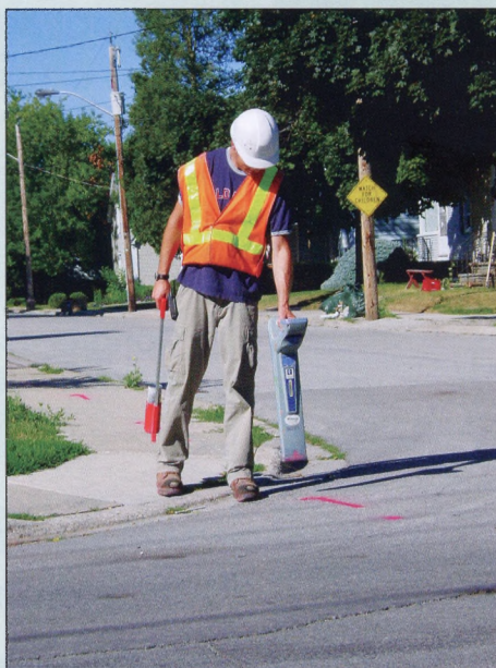
Figure 1: Electronic line locators are commonly used to define the routing of underground metallic utilities.
